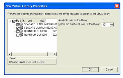
**Note:** The slot range specified is in sequential order, beginning with the first slot in the library. Make sure that you select the drives having the same media type as the media in the first slot range.
