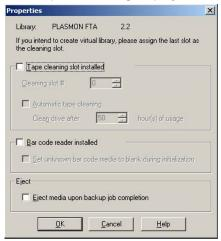
The Properties dialog allows you to specify which slot holds the cleaning media (if present) and whether a bar code reader is installed.
